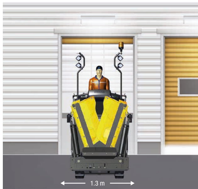
Transport width 1.3 m. Fits through any space that a 4.5 t forklift can pass through.
